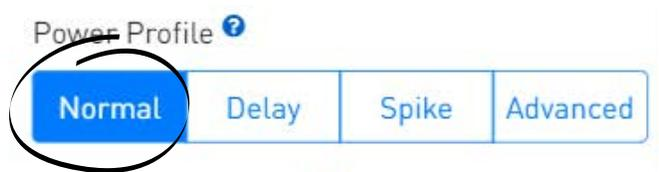
Tools that roar to life as soon as they are powered on have a "Normal" power profile. To properly configure this type of tool, look at its power graph.
