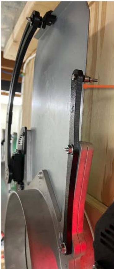
The slide of the metal blast gate will glide along the metal bearings of the Slide Guide to keep it on track.
