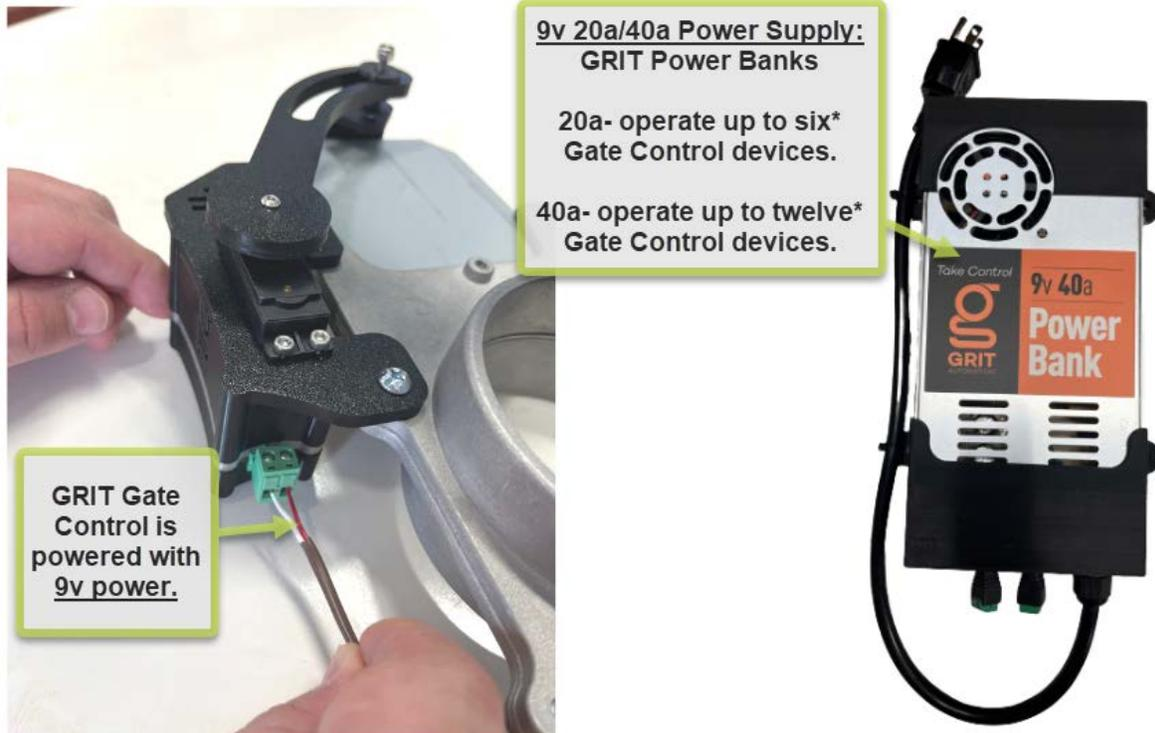
The low-voltage wire can be run from a device to the Power Bank in a "home run" fashion, or, hopped from one Gate Control device to the next on its way to the Power Bank in a "daisy chained" fashion. The Power Bank has two low-voltage jacks, but two sets of wires can be landed in each, if needed.
